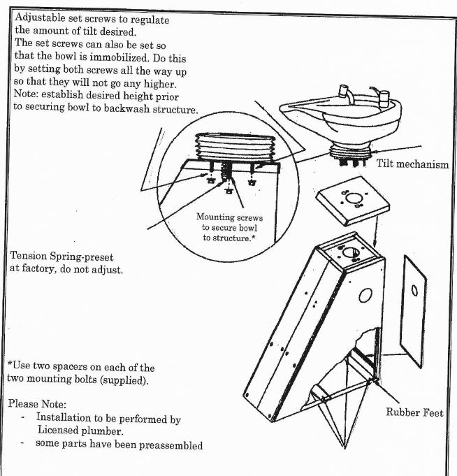
Holes for mounting structure to the ground
